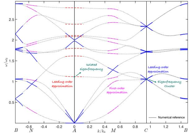
Figure 2: Approximation of the first twelve dispersion branches for the Miura-ori periodic structure.
