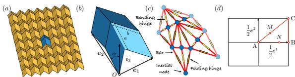
Figure 1: (a) Truncated 2D periodic Miura-ori sheet (b) unit cell of periodicity, (c) discretized unit cell, and (d) first BZ of the lattice.
