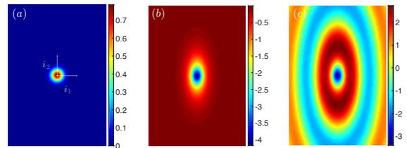
Figure 3: (a) Amplitude of the driving force and corresponding leading-order approximation of the induced effective motion within: (b) band gap, and (c) pass band near the origin of the first BZ.
