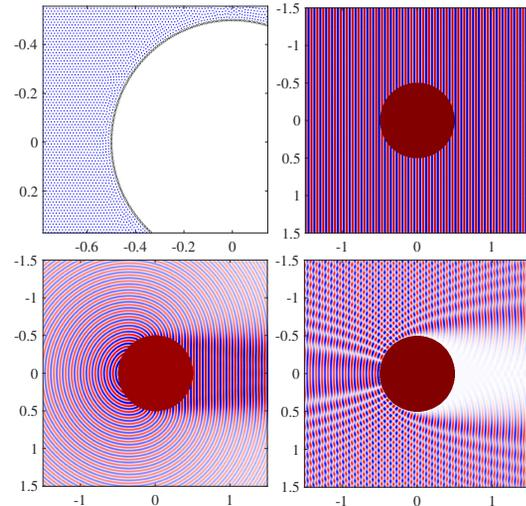
Figure 1: Top left: Distribution of nodes surrounding a circular obstacle  $\Omega_{obs}$ . Top right: Incident wave field  $u_{inc}$ . Bottom left: Numerical solution of the scattered wave field  $u_{sct}$ . Bottom right: Total wave field  $u = u_{inc} + u_{sct}$ .
