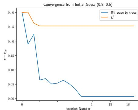
Figure 3: Convergence to global minimum for  $W_2$  versus convergence to local minimum for  $L^2$
