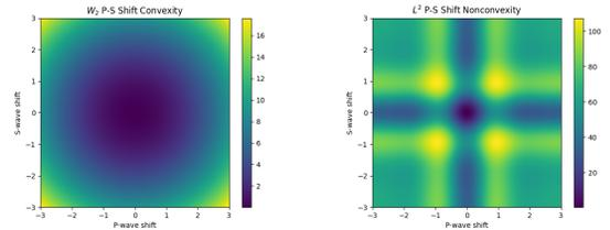
Figure 1: Comparison of optimization landscape of  $W_2$  and  $L^2$  distances for elastic waves that have been shifted away from origin according to varying  $P$  and  $S$ -wave velocity differences.
