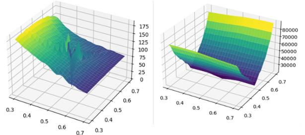
Figure 2: (left)  $L^2$  squared distance v. source location, (right)  $W_2^2$  v. source location. Synthetic data generated from source location at center of domain  $(0.5, 0.5)$ , where global minimum is located.
