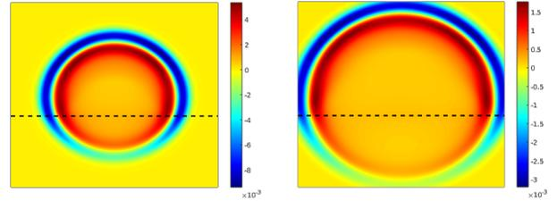
Figure 2: Pressure of the acoustic wave with the absorption coefficient  $\sigma = 7$ , on the left at  $t = 0.31$ s and on the right at  $t = 0.47$ s.
