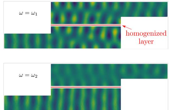
Figure 3: Effects of suppressing the acoustic field for some frequencies (here for  $\omega_2$ ) inducing the metasurface behaviour.
