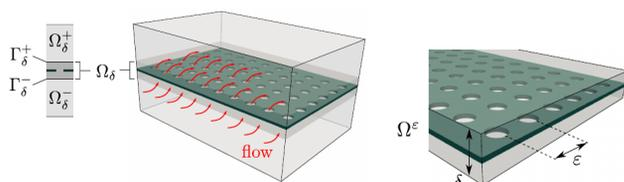
Figure 1: Thin layer with a perforated plate
